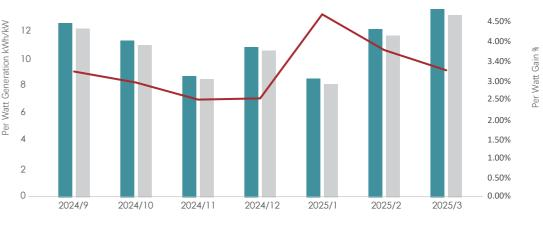
Jinko TOPCon Per Watt Generation P-type BC Per Watt Generation — Per Watt Gain
